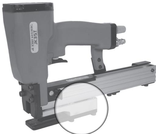
During operation, the pliers' gap is fixed. If necessary the gap can be set to accommodate different material thicknesses. Spacers with 3 and 6 mm thickness are available. These spacers are delivered with the tool, together with a set of longer screws to be used when spacers of more than 3 mm total are inserted.
